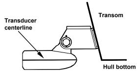
Align transducer centerline with hull bottom.
